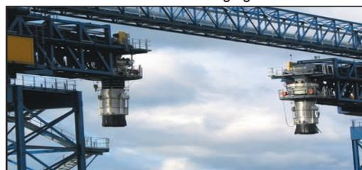
*Stockpiling of coal with use of a tripper conveyor.*
