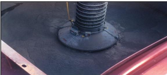
Ship loading spouts utilizing compact filter modules
