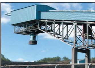
*OV style heavy duty loading spouts with compact filter modules on swinging boom.*
