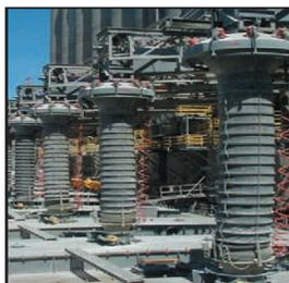
Model OV44 loading spout with model CFM470 loading kaolin clay.
