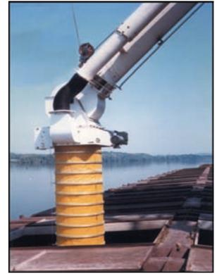
Pivoting gimbal allows different loading angles.
